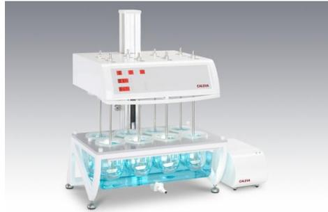
The high standard dissolution tester CALEVA 11+ST guarantees an easy and comfortable access with its individual display for each test-run parameter (time, rpm, temperature) and UP/DOWN buttons for fast and easy test-run parameter settings. For better observation of the sample dissolving process the one-piece moulded water bath (with standard water outlet cock) is illuminated (optional).
