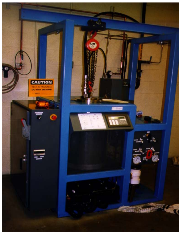
FIGURE 3. A 20-LITER EXTRACTION VESSEL UNIT (SFT, INC.) SCALE UP WORK
